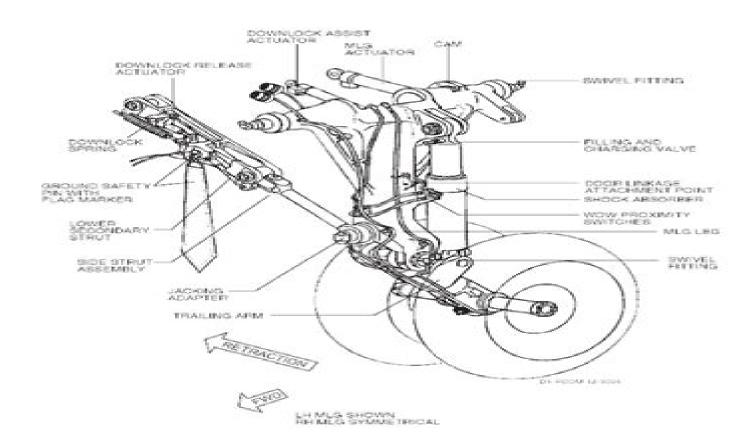
Main Landing Gear Assembly (LH Side Shown)
